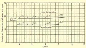
Fig. 266A.—Graphs showing water rates of a Skinner 21 in. × 22 in. uniflow engine running non-condensing and condensing, saturated steam at 140 lb. (This and the next illustration are from data on engines which were direct-connected to generators of 200 true kw. capacity and would be considered 320 h.p. engines at normal full load. However, the engines are good for 400 indicated h.p. for maximum continuous operation.)
